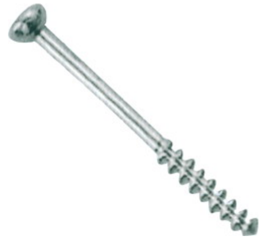
ORTHOPEDIC IMPLANTS JKA-332.45 Cancellous Screw 6.5mmx32mm Thread 45 mm,
